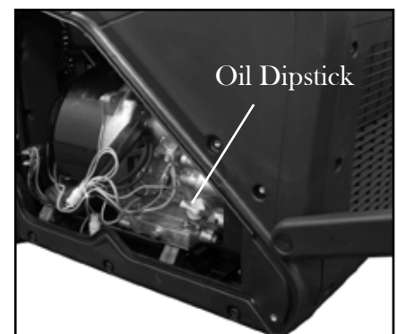
Fig. 2 - Oil Fill Opening, Dipstick and Oil Level
